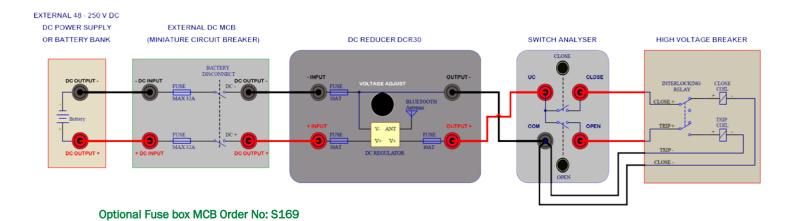
The output voltage can be adjusted in two ways; With the integrated digital voltage adjustment knob.
