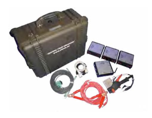
All kits come complete with system software BTS11 with free upgrades, manuals, main cable, communication cable, connection accessories, soft cable bag and free support.
